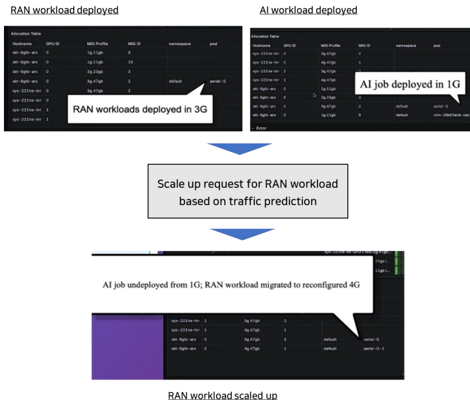
Figure 7. Test result for GPU reconfiguration
